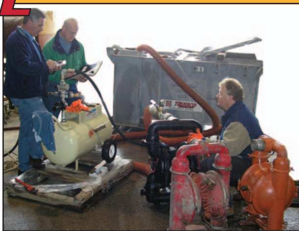
FIGURE 4. MATT BRIGNAC (AGI), LYLE SHOUP (INGERSOLL RAND) AND BILL O'TOOLE (AGI) CONDUCT AN ON-SITE, SIDE-BY-SIDE AIR CONSUMPTION COMPARISON OF ARO EXP AND EXISTING DIAPHRAGM PUMPS. (INGERSOLL RAND)
