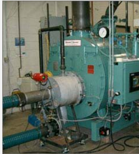
Prototype "Super Boiler" uses a two-stage, firetube design that is compact and efficient.
